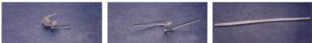
Figure 2. Material metamorphosis: when heated, biodegradable shape-memory polymer transforms from a temporary shape (left) to its parent shape (right) within 20 seconds.
